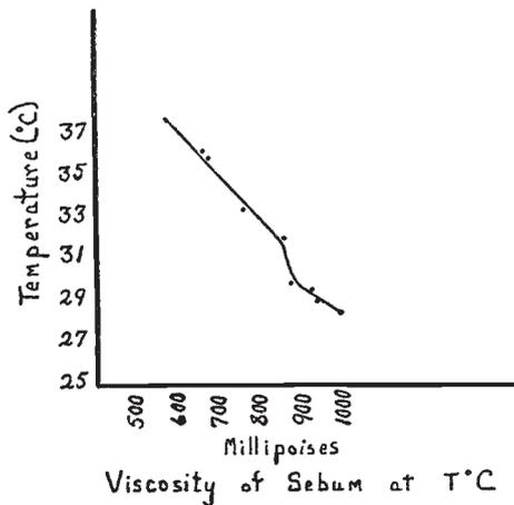
In studying the figures in table 2 it will be seen that the time of flow per degree centigrade is relatively small up to 30° C. and much greater beyond that point. The average overall time of flow between 38° and 30° is seen to be 9.8 seconds/°C., and from 30° to 26.5° it is 23.7 seconds/°C.
